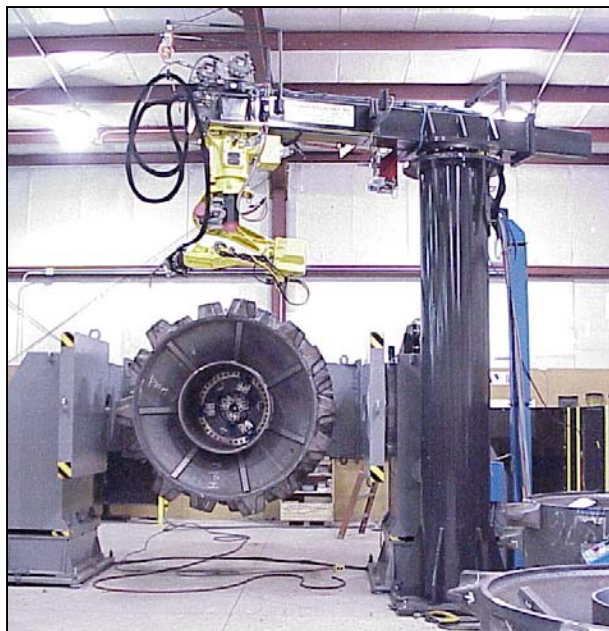
Robotic swing boom positioner shown integrated into weld system with FANUC Robotics Arcmate 120i and part positioner
