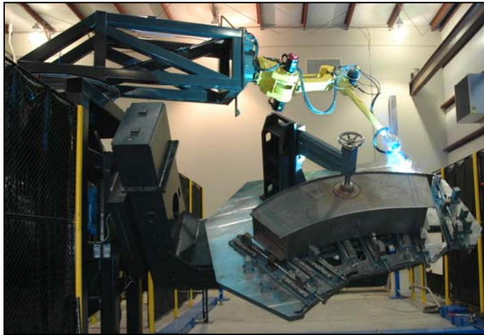
Welding application with custom fixtures
